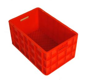
Crate is made of virgin HDPE. Base of the crate is specially designed for higher load bearing capacity and continuous ruggedness on the factory floor. Thickness of crate base is 19 mm (7 mm ribs on each side + 5 mm base) instead of 7 mm in regular crates( 4 mm base + 3 mm outside ribs). The base thickness is 2.5 times more compared to the standard crates which will certainly increase the life of the crates. Crates are 20-25% heavier than other crates of same dimensions.
