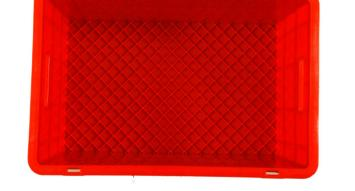
In order to strengthen the crate our design has checkered ribs of 7 mm height at 25.4 mm distance between two consecutive ribs so that the any object does not touch the crate base directly. Hence specially designed checkered ribs act as protection to the base adding longer life to the crates.
